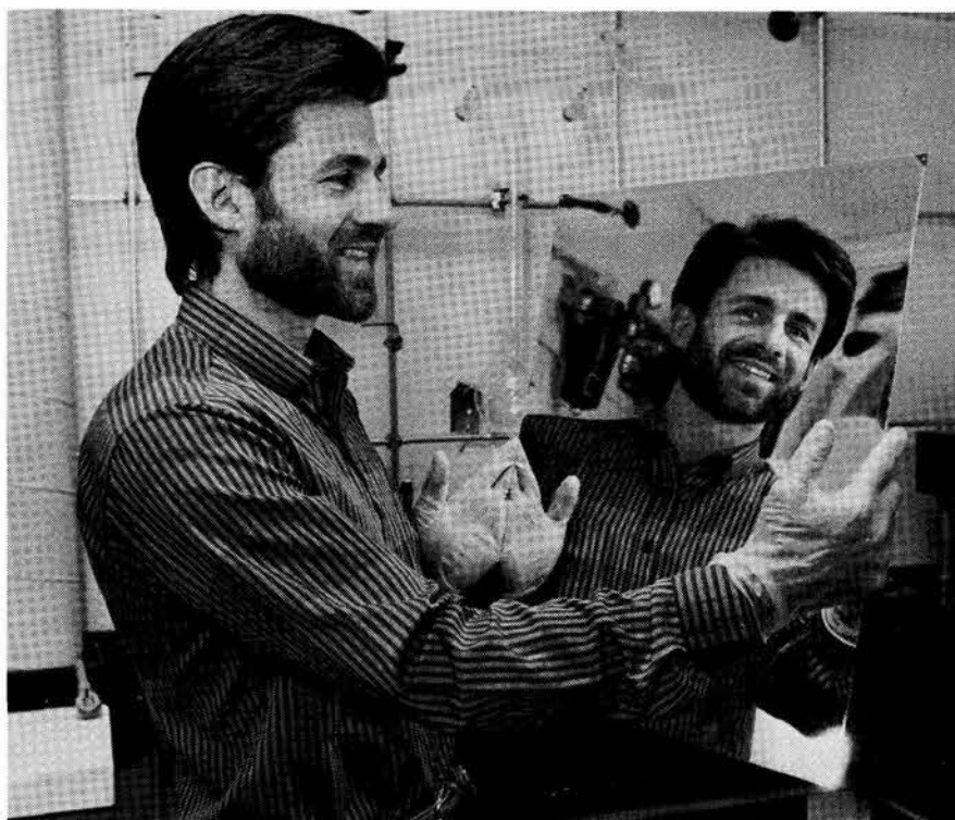
JEFF BRINKER (1846) displays mirrored stainless steel substrate created through a sol-gel process. This unit is part of the flexible solar mirror project; the work to achieve the increased size of such mirrors was done by Carol Ashley (1846) and Scott Reed (7471).
